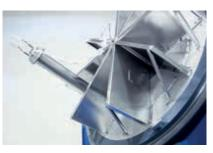
engine turbo pumps. The anti-vortex device minimizes unusable propellant mass.
