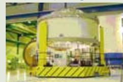
ESC-A\*: liquid oxygen tank
