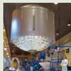
EPC\*\*: liquid hydrogen and oxygen tanks
