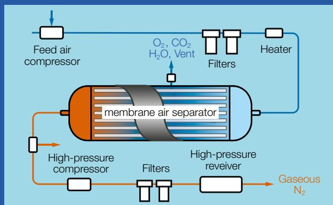
The GENA 20 nitrogen generator is a fixed and compact high-purity (residual oxygen 2%) and high-pressure (300 bar - 4350 PSI) inert gas production unit.
