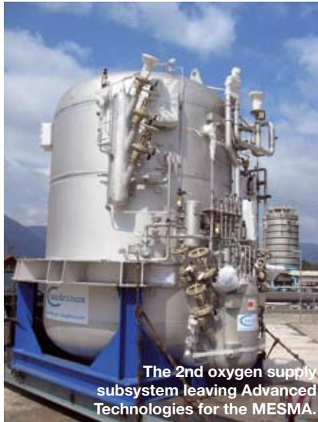
The 2nd oxygen supply subsystem leaving Advanced Technologies for the MESMA.
