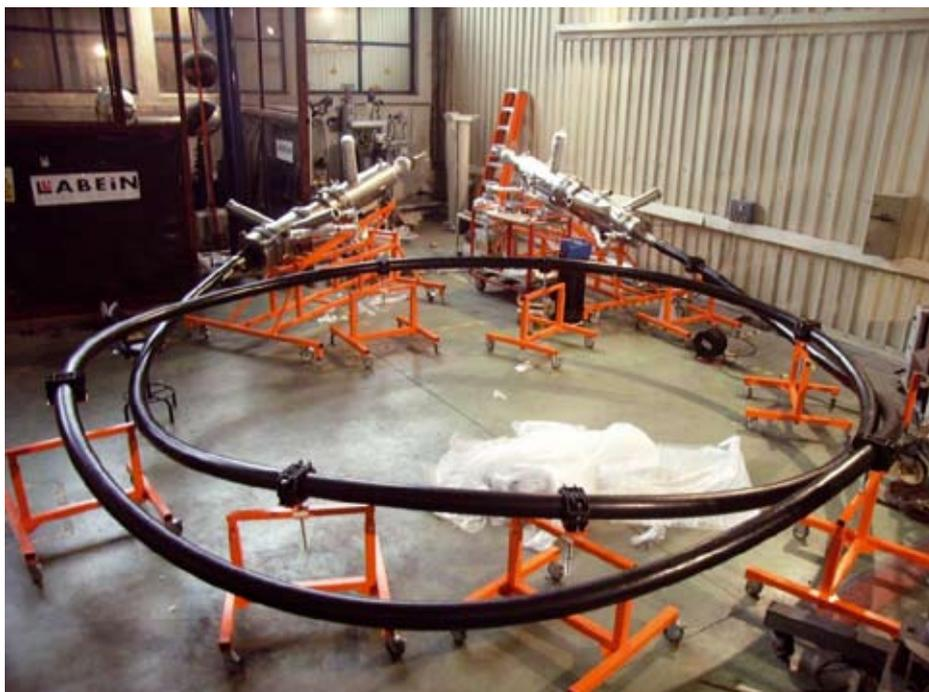
**In Bilbao, Air Liquide Advanced Technologies delivered a cooling unit used to cool the Super 3C cable, shown here in the workshop with the two cryostats at either end.**
