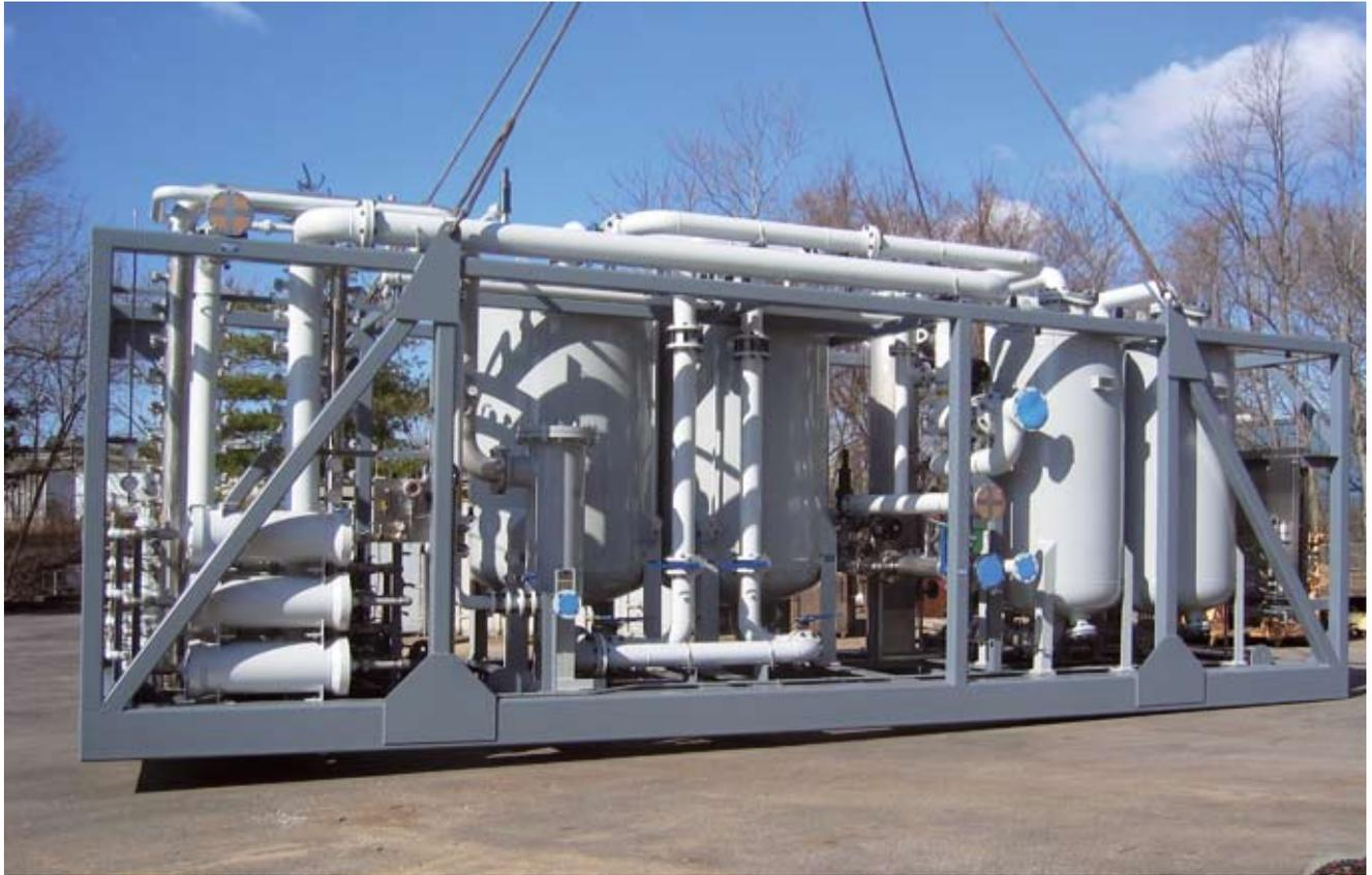
**On the left: the double-stage membrane system serving to eliminate carbon dioxide. In the centre: the PSA (Pressure Swing Adsorption) module. On the right: the two columns of activated charcoal used to eliminate VOCs, siloxanes and hydrocarbons.**
