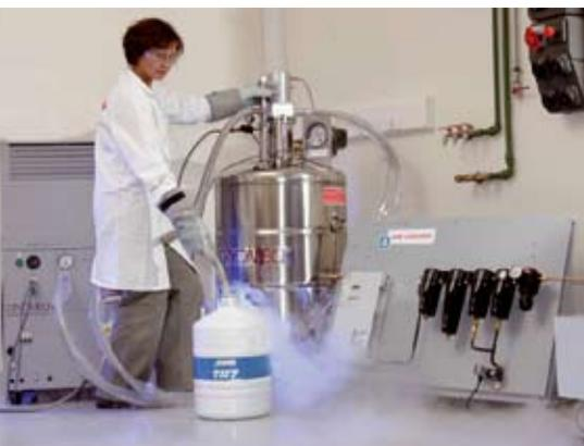
**The LNP particularly contains a cryogenic coolant based on Gifford-MacMahon technology produced by Cryomech (Syracuse, New York).**
