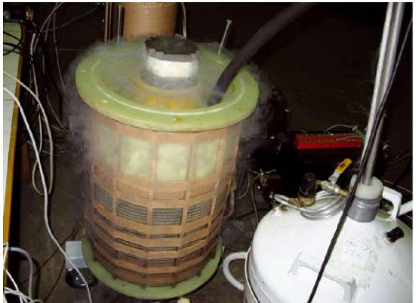
This 20 kVA cryostat delivered to Budapest is made of composite material (epoxy glass). A second one of 100 kVA will soon be completed.
