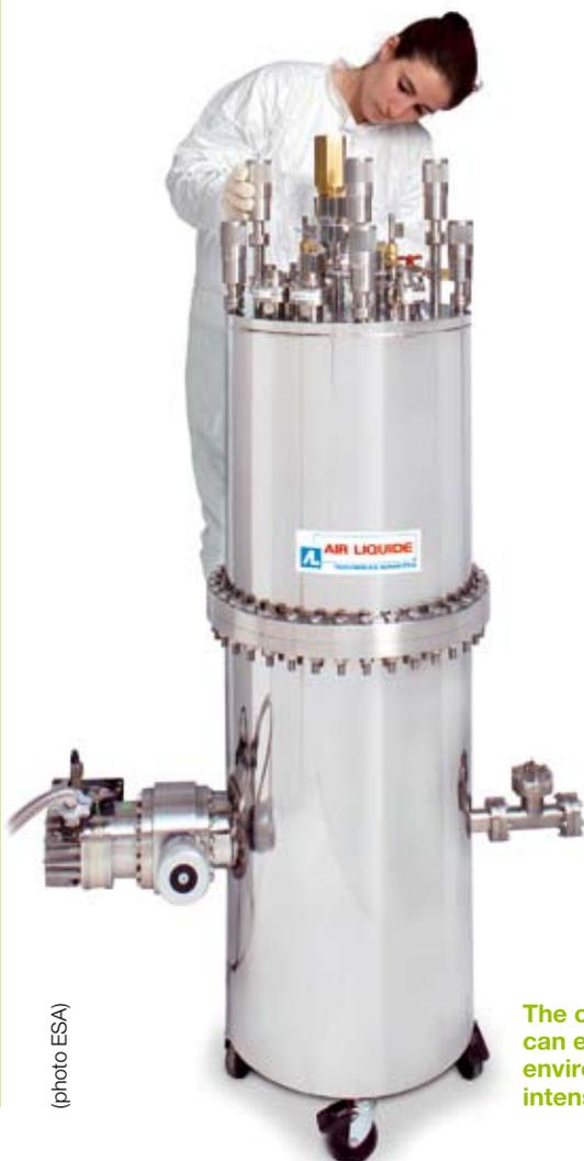
The cryostat at the University of Taiwan can examine samples at 300 mK, in a UHV environment (10<sup>-10</sup> millibars) and a very intense magnetic field (7 tesla).
