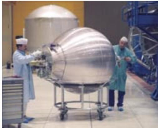
**The Liquid Helium SubSystem which will pressurize the main stage oxygen tank in the next thirty Ariane launchers.**
