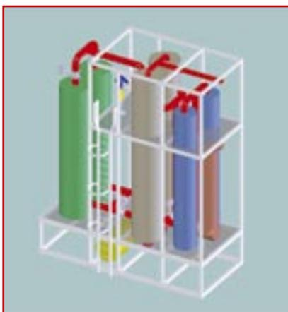
Diagram of the DTA installation for Finorga. The Finorga installation breaks down into four stages – in pink, the first stage; in blue, the second stage; in grey, the third stage; in green, the fourth stage; and in yellow, the recovery tank.
